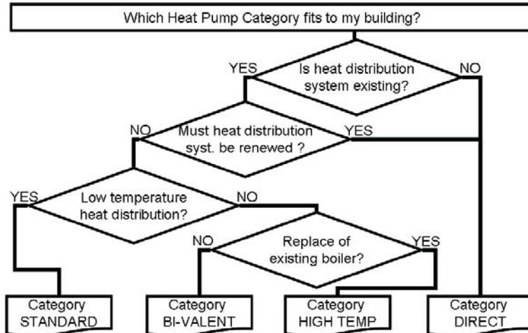
A selection chart was developed to distinguish between different types, in which case a type of heat pump can be used and which assumptions a building should fulfil.
